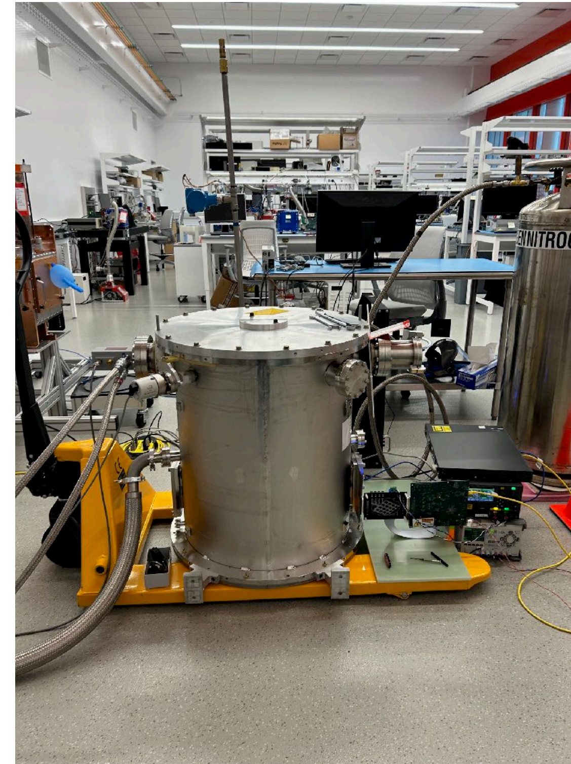
3 MCMs operating in nitrogen gas (15 PSI). This is a test of the MIDNAs + operations in gas. Can have up to ~200 CCDs
