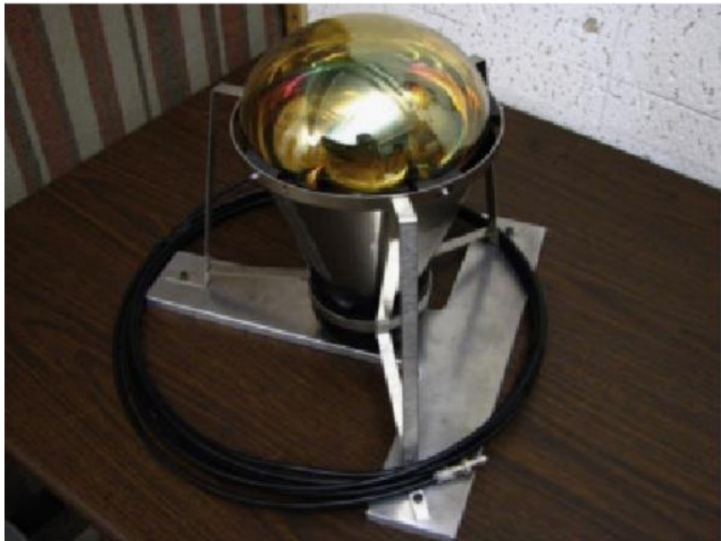
PMT assembly (nEXO Pre- Conceptual Design Report)
