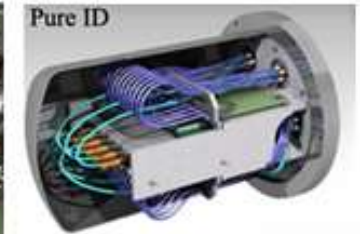
Underwater electronics: Case design and feedthrough
