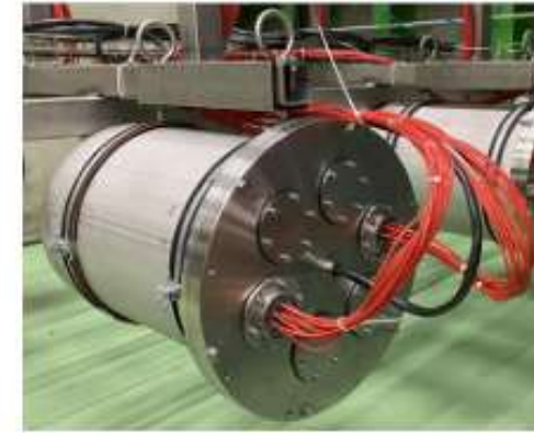
Underwater electronics: Case design and feedthrough
