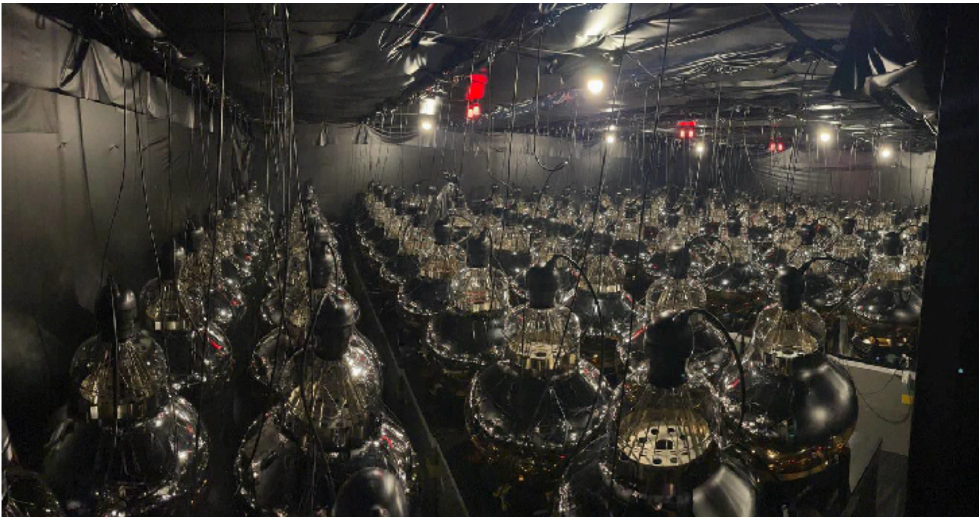
▶ Mass QA testing of 200 PMTs
