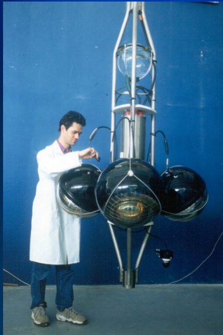
Assembly of one ANTARES 'storey'
