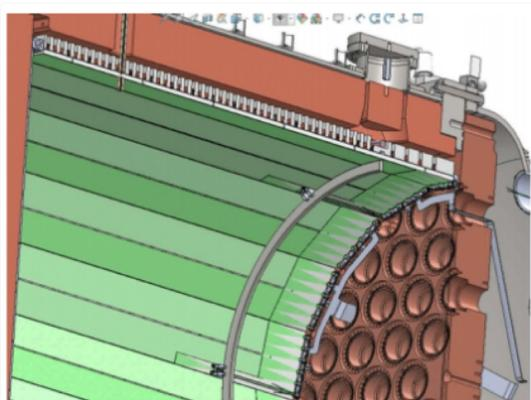
Barrel Fibre detector readout for energy readout
