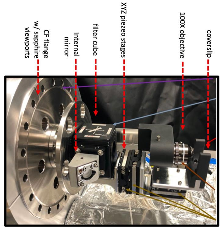
Microscope has a  $5 \times 5 \text{mm}^2$  scan area with  $1 \times 1 \text{mm}^2$  scan area demonstrated at pressure
