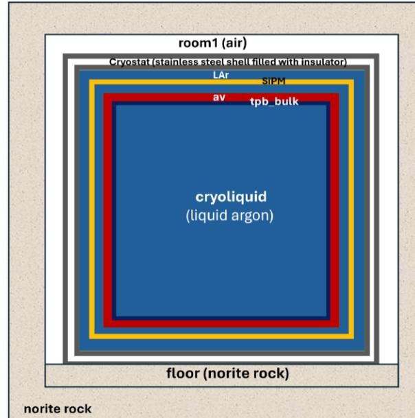
2-D cross-section of detector components
