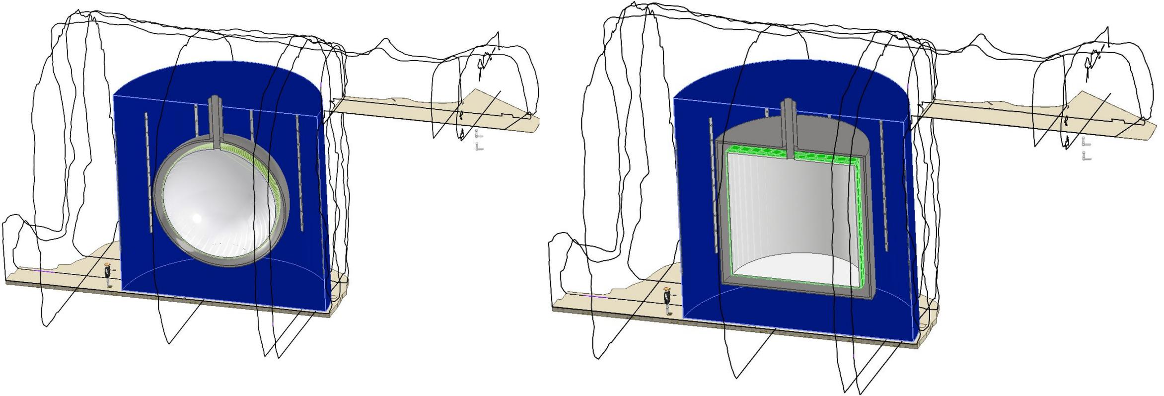
Increase inner dimension to reduce neutron backgrounds within fiducial volume; change protoDUNE-style cryostat to vacuum cryostat + large water shield to reduce external neutrons.
