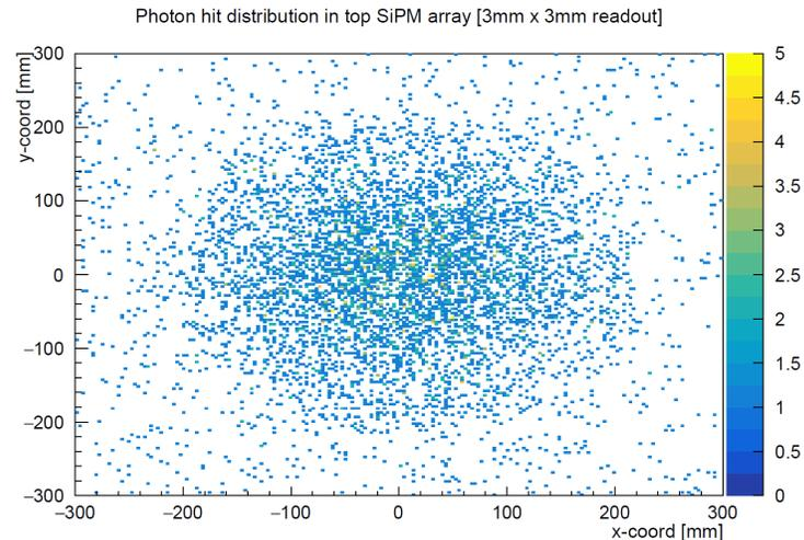
Left: hit pattern imaged onto pixelated photodetectors over 60x60 cm<sup>2</sup> area for surface events. Developing hit-pattern ID algorithms.
