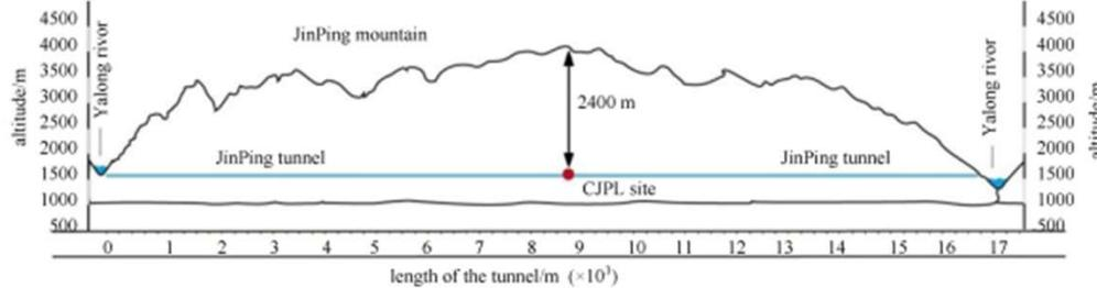
Fig. 1. Cross section of Jinping mountain and location of the CJPL.
