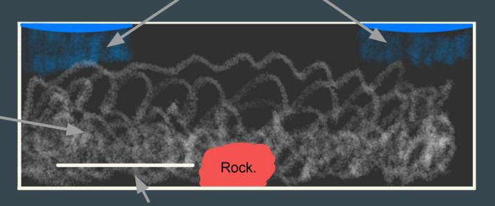
The subatomic particle ionizes some of these alcohol atoms, leaving an electric field, attracting more dipoles and creating a visible contrail
