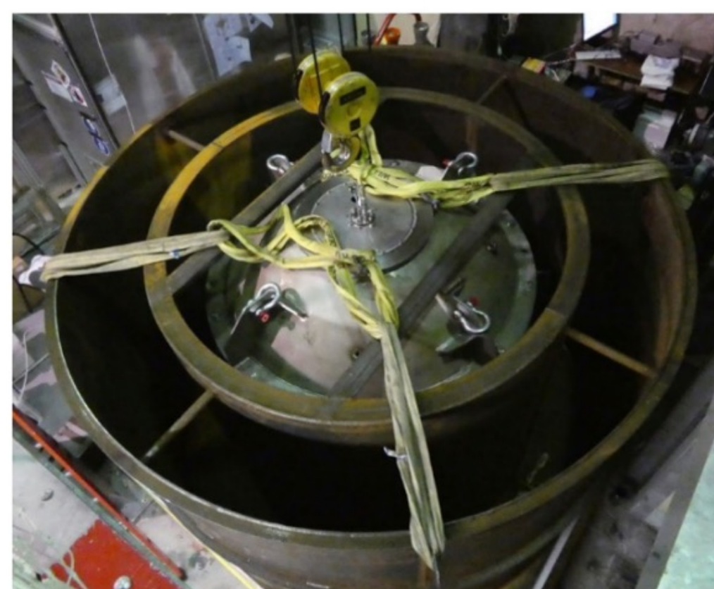
Sphere in Pb shield installed in temporary water shield in summer 2019
