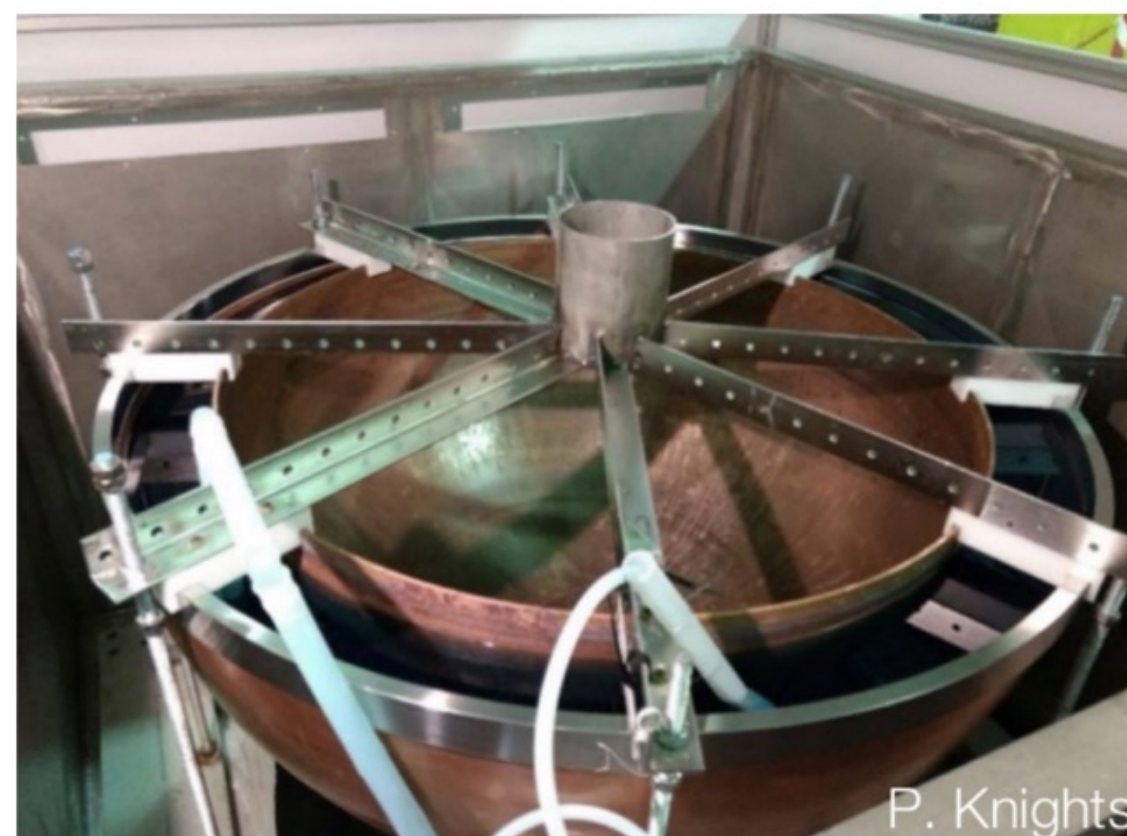
0.5 mm copper plating on hemispheres at LSM to manage 210 Pb in copper bulk
