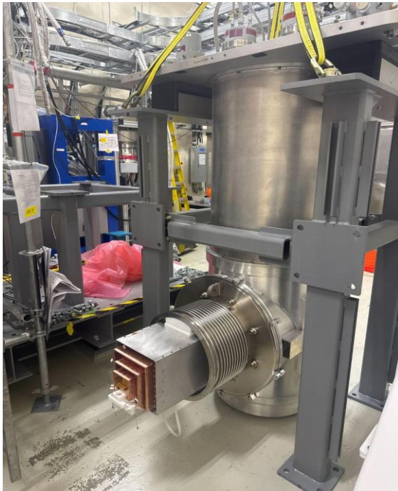
Dilution fridge with cryogenic tails, just prior to its installation
