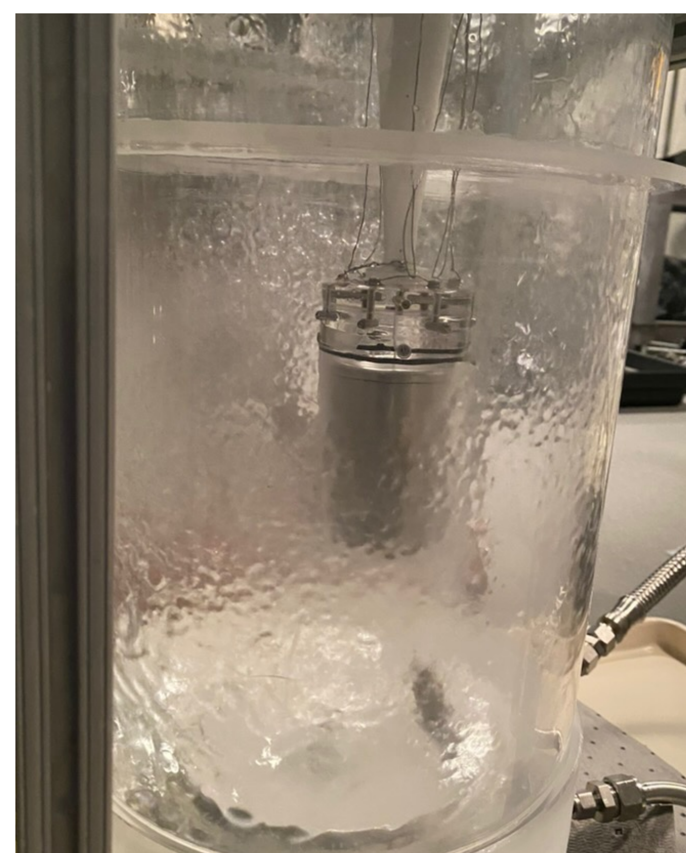
SNO+ Americium-Beryllium (AmBe) source inside the Source Cleaning Vessel (SCV)
