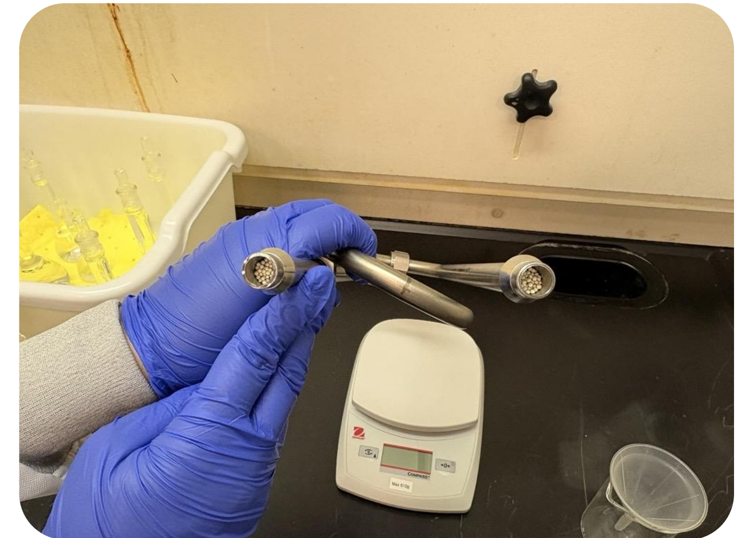
Filled trap with ~85g of Zeolite
