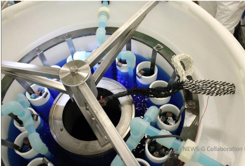
The ECA electroforming bath at PNNL
