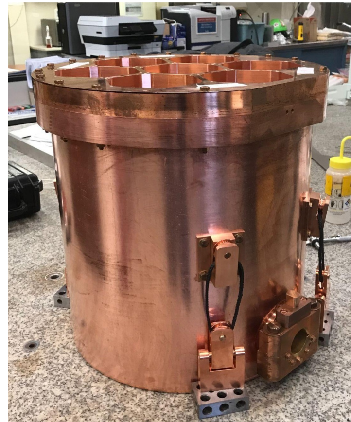
Pre-assembled chamber, hanger brackets, clamps and tower lid Verified hanger clamp location
