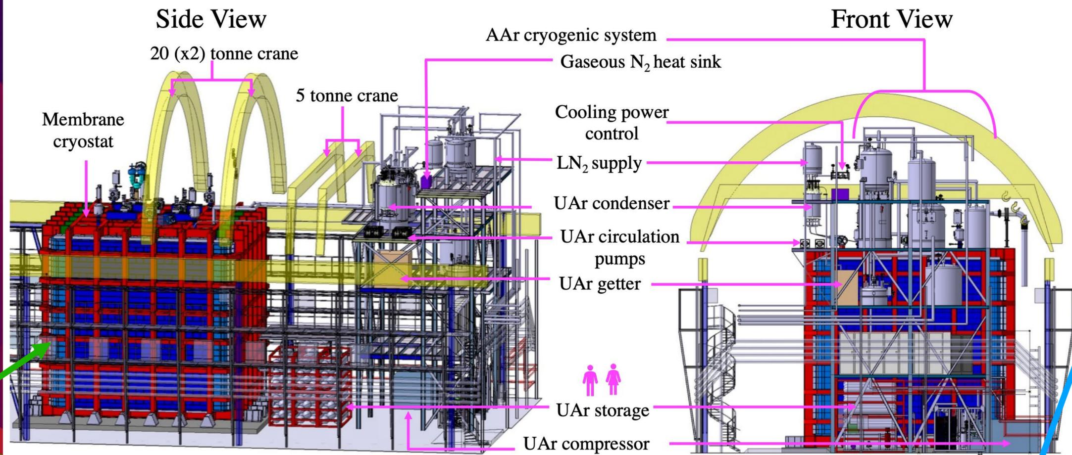
DUNE-like membrane cryostat
