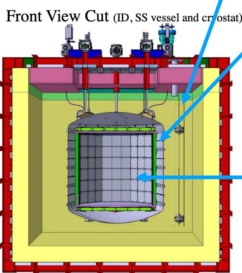
50 tonne (20 tonne fid.) underground argon volume dark matter target
